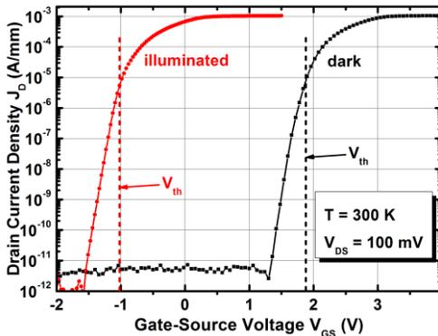
Fig. 1: Normally-off transfer characteristics of an FET fabricated from a GaN/AlGaN heterostructure without a conductive channel at 300 K in the dark. A channel is formed under UV exposure, which results in normally-on FET operation.
