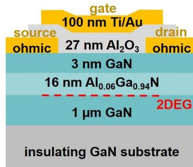
Fig. 4: Cross-sectional illustration of a lateral FET fabricated from a GaN/AlGaN heterostructure with no 2DEG present in the dark. The overlap of gate and source/drain contacts is essential for FET operation, since only underneath the gate electrode a 2DEG can be generated electrostatically. Gate and source/drain contacts are separated by a highly insulating dielectric layer.
