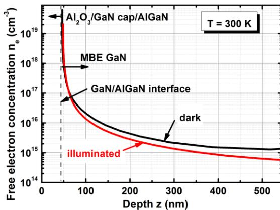
Fig. 5: Vertical free electron density profiles extracted from capacitance vs. voltage measurements. For both cases of optical and electrostatic generation, the conductive 2D channel is located at the GaN/AlGaN interface.
