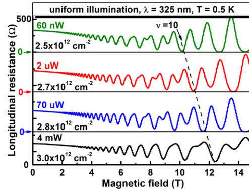
Fig. 2: Low temperature longitudinal magneto-resistance of a Hall bar device under steady UV excitation at different power. An increase in the illumination power of almost 5 orders in magnitude only raises the channel density by 20 %.
