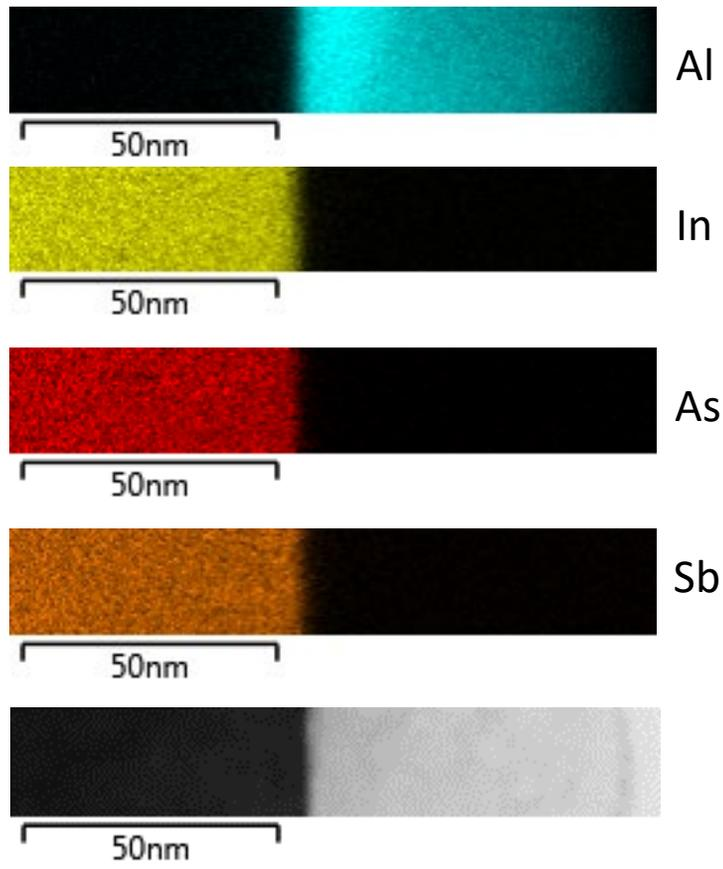
Figure S3 Energy-dispersive spectroscopy map of Al – InAsSb interface.
