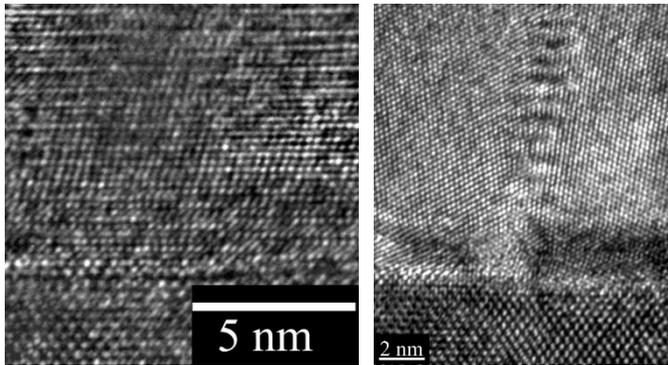
Figure 1. (left) Interface between AlSb intermediate layer and Al. (right) Interface between InAsSb and Al with no intermediate layer.
