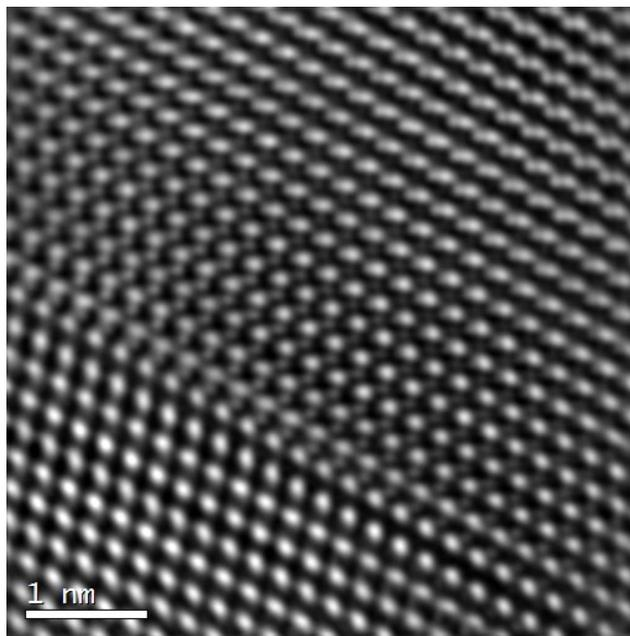
Figure S2. TEM image of twinned Al film grown on InAsSb.
