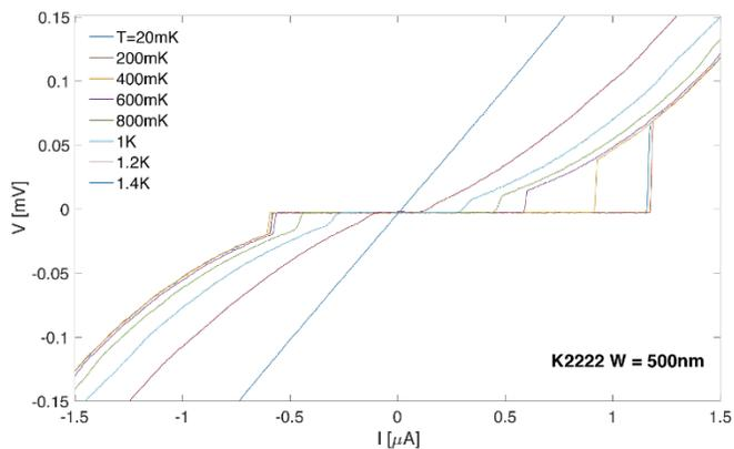
Figure S1. The current-voltage characteristics of Josephson junctions fabricated on our Al-InAsSb materials shows supercurrent. The temperature dependence of the supercurrent suggests high interface contact transparency.
