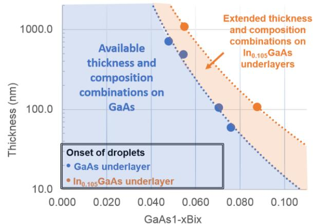
Fig 1: GaAs<sub>1-x</sub>Bi<sub>x</sub> epilayer thickness as a function of bismuth composition for samples grown on GaAs underlayers (blue) and In<sub>0.105</sub>GaAs underlayers (orange).
