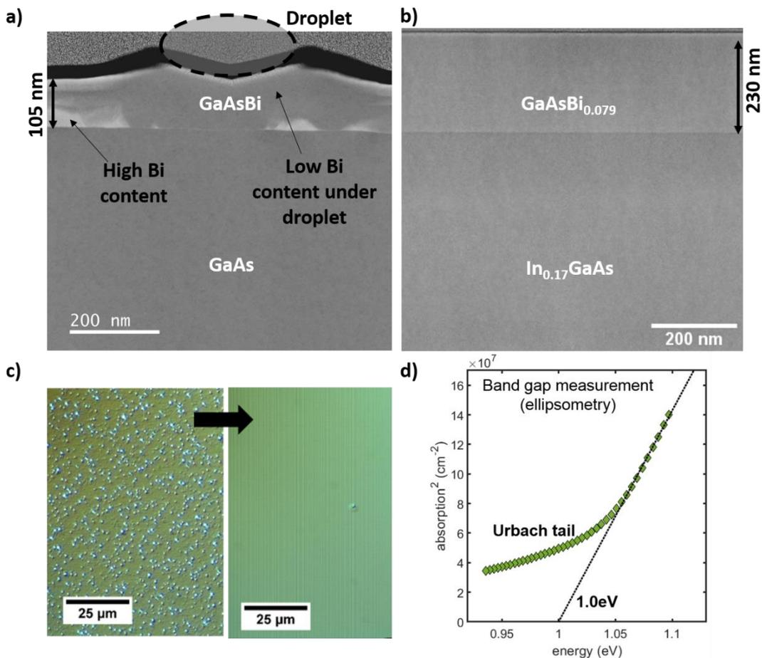
(a) HAADF STEM image of Bi saturated GaAsBi sample. Ga-Bi droplet formation on the surface leads to both lateral and vertical phase separation. Specifically, in regions directly underneath the droplets the Bi content is significantly reduced due to Bi incorporation into the droplets, and the growth rate is enhanced due to excess Ga atoms from droplets.
