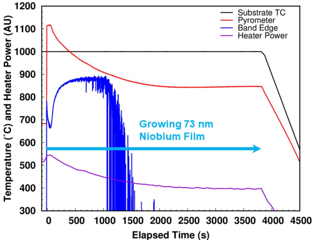
Measured temperature and power excursions for 73 nm niobium (Nb) film grown on transparent Si 4H-SiC substrate with fixed heater thermocouple (TC) temperature illustrating:
