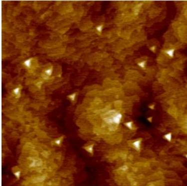
$2 \times 2 \mu\text{m}^2$  AFM images of tensile-strained (top) 0.6 BL Ge and (bottom) 4.5 ML GaAs QDs. We grew both samples at 535 °C. The top and bottom images have a z-scalebar of 1.5 nm and 4 nm, respectively.
