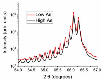
Figure 1: X-ray diffraction spectra from two superlattice samples of InAs/GaAs SMLQDs grown with high and low arsenic fluxes.
