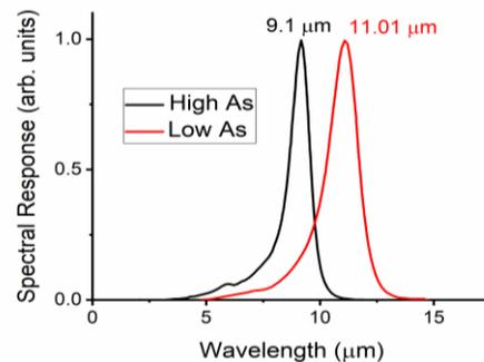
Figure 2: Spectral response at 10 K of two SML-QD superlattice samples grown with high and low As fluxes.
