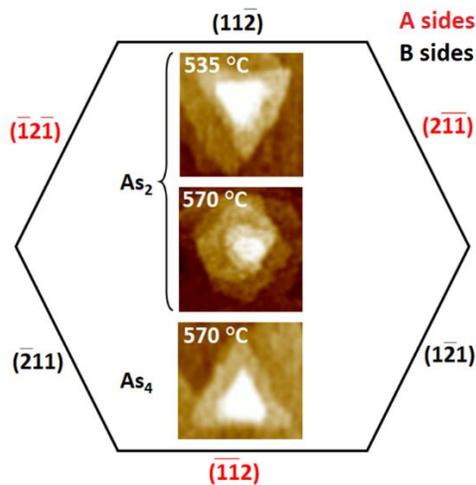
Fig. 4. AFM images of the various GaAs(111)A TSQD morphologies with different substrate temperature and arsenic species combinations. Overlaid is a schematic of the  $\{211\}$  planes relative to the possible TSQD step edge orientations.
