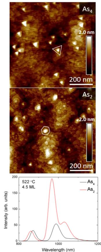
Fig. 1. AFM of triangular (a) and hexagonal (b) TSQDs. Brighter TSQD PL with As<sub>2</sub> (c).
