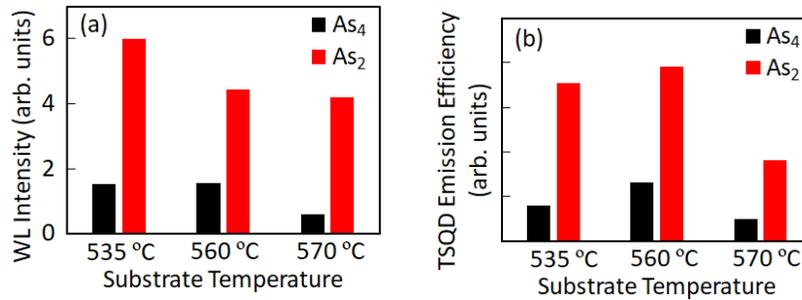
Fig. 3. Plots of GaAs(111)A WL emission intensity (a) and TSQDs emission efficiency (b) with increasing substrate temperature. WL intensity and TSQD emission efficiency are higher consistently higher with  $As_2$  than  $As_4$ .
