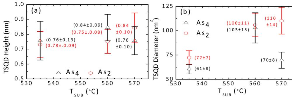
Fig. 2. Scatter plots of the average (a) height and (b) diameter of TSQDs grown with  $As_4$  (black) and  $As_2$  (red), as a function of substrate temperature (error bars represent one standard deviations).
