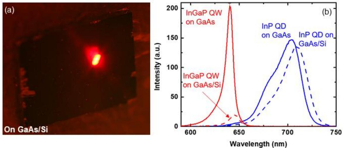
Figure 4: (a) Photo of PL from InP QDs on GaAs/Si at RT with green laser filtered out, sample size =  $1.5 \text{ cm} \times 2 \text{ cm}$  (b) PL of InP QDs on GaAs/Si and GaAs showing similar integrated intensity and far greater dislocation tolerance compared to InGaP QWs.
