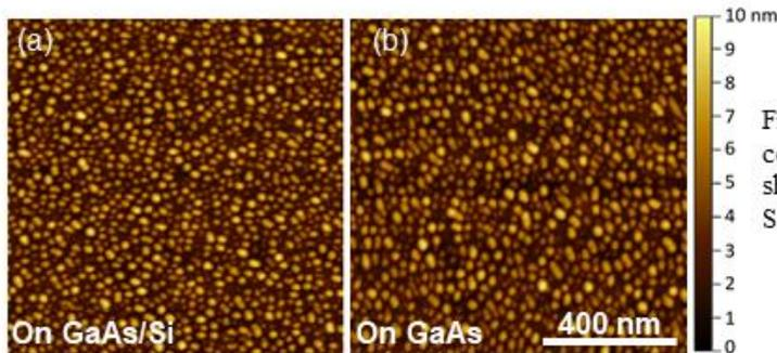
Figure 3: AFM of 3 ML InP QDs simultaneously co-grown on (a) GaAs/Si and (b) GaAs. Both show very high dot density of  $\sim 1.3 \times 10^{11} \text{ cm}^{-2}$ . Same scale bar for (a) and (b).
