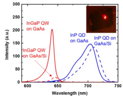
Figure 1: PL of InP QDs on GaAs/Si and GaAs showing similar integrated intensity and far greater dislocation tolerance compared to InGaP QWs. (inset: photo of PL from InP QDs/Si with green laser filtered out, sample size = 1.5 cm  $\times$  2 cm)
