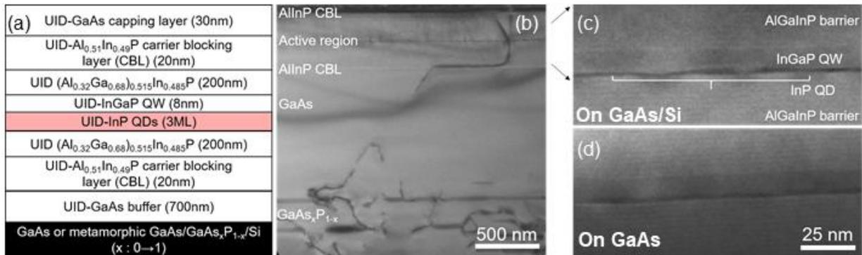
Figure 1: (a) InP QD structure for PL experiments, (b) Low- and (c) high-magnification XTEM image of InP QD active region on GaAs/Si. (d) XTEM of active region on GaAs showing nearly identical morphology. (b) taken with  $g = \langle 004 \rangle$  and (c)-(d) taken with  $g = \langle 002 \rangle$  two-beam conditions. Same scale bar for (c) and (d).
