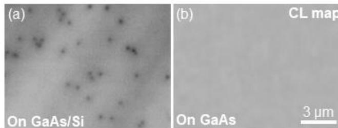
Figure 2: CL image of InP QD active region co-grown on (a) GaAs/Si showing TDD =  $3.3 \times 10^7 \text{ cm}^{-2}$  (dark spots), and (b) GaAs. Same scale bar for (a) and (b).
