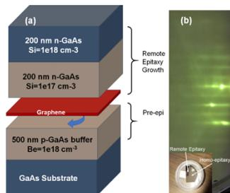
**Figure 1:** (a) Heterostructure of the graphene/III-V heterostructure hybrid diode; (b) RHEED image of the GaAs during the remote epitaxy growth: inset: micrograph image after growth
