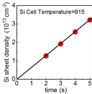
Fig.9 Si sheet density vs shutter time (s)
