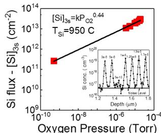
Fig.4 Si flux vs O<sub>2</sub> pressure
