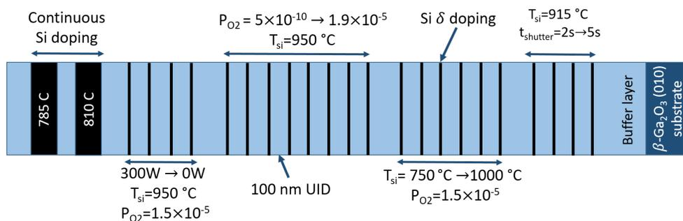
Fig.8 Epitaxial structure used for SIMS analysis (All pressures are in units of Torr)
