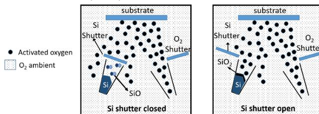
Fig.2 SiO and SiO<sub>2</sub> formation inside MBE chamber
