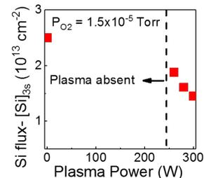
Fig.5 Si flux vs plasma power
