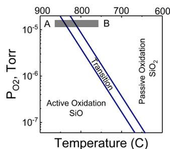
Fig.7 Si-O P-T diagram [2]
