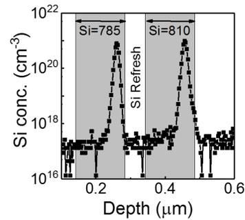
Fig.10 Si sheet density for extended shutter time
