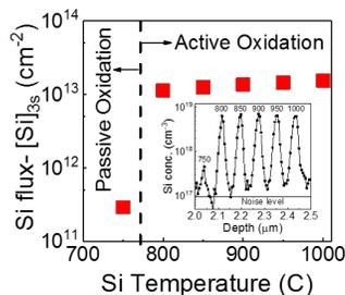
Fig.3 Si flux vs Temperature
