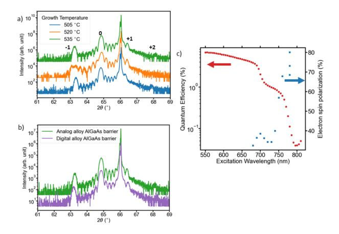
Initial characterization of strained superlattice InAlGaAs/AlGaAs photocathode structures grown pseudomorphically on GaAs(001)
