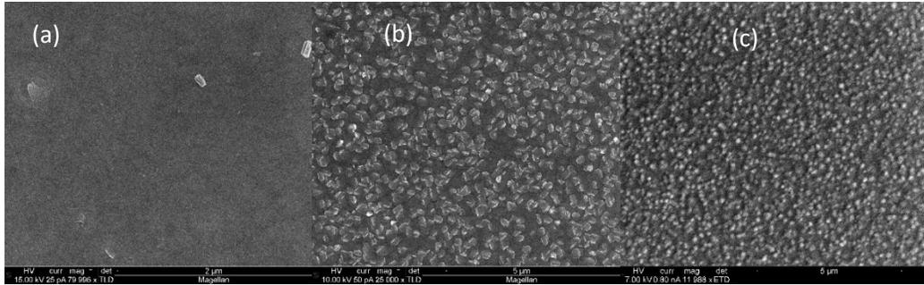
Fig. 1 SEM images of  $\text{Ge}_{0.84}\text{In}_{0.16}\text{Te}$  (a),  $\text{Ge}_{0.81}\text{In}_{0.19}\text{Te}$  (b) and  $\text{Ge}_{0.60}\text{In}_{0.40}\text{Te}$  (c) films.
