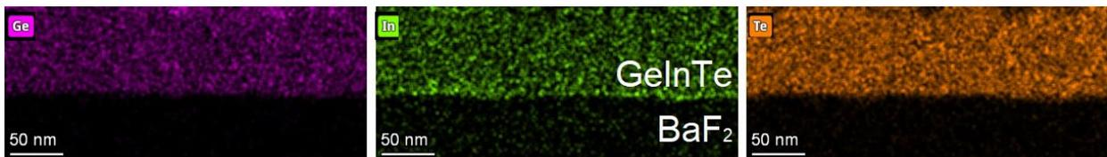
Fig. 4 Energy dispersive X-ray (EDX) mapping analysis of composites at  $\text{GeInTe}/\text{BaF}_2(111)$  interface.
