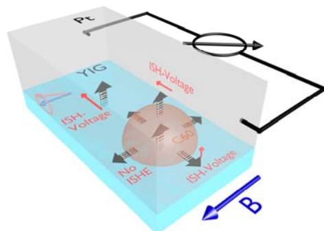
Figure 2: Sketch of the ISHE resulting from spin currents flowing from YIG into Pt through a  $C_{60}$  half-sphere
