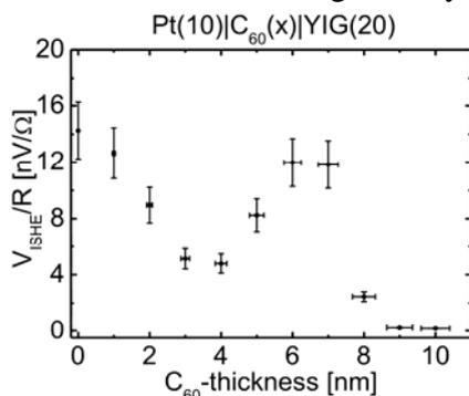
Figure 1: Dependence of ISHE on  $C_{60}$  interlayer thickness  $d_0$
