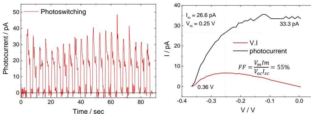
Figure: Demonstration of photodetector and photovoltaic application. Photoswitching experiment of the diode was performed at 0 V under 638 nm illumination. The fill factor of the diode was determined to be 0.55 under 638 nm illumination.
