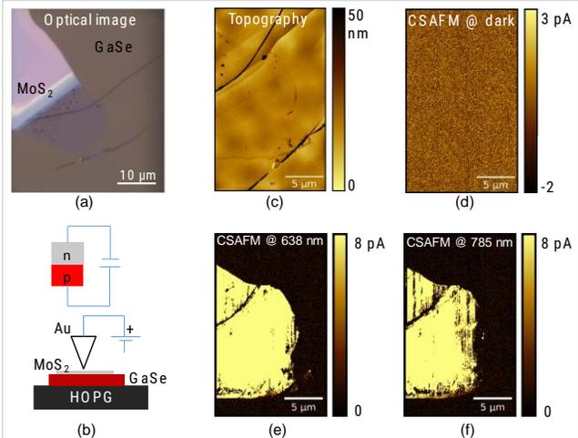
Figure: GaSe/MoS<sub>2</sub> p-n junction. (a) optical image of the heterostructure, (b) schematic of the device and experiment, (c) AFM topography of the diode, and (d) – (f) CSAFM images of the diode in the dark and illumination
