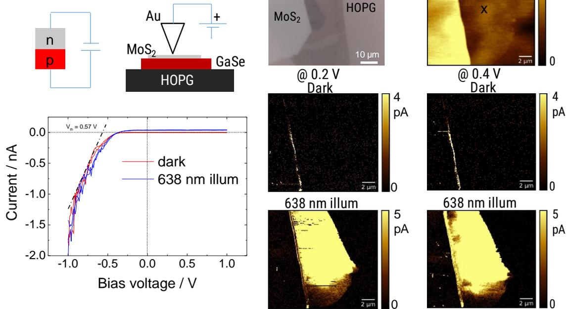
Figure: Demonstration of the formation of p-n junction in ultra-thin van der Waals vertical heterostructure. The schematic of the device and the experimental configuration (top left). Optical image of the heterostructure and the AFM topography (top right). The I – V curves in the dark and illumination taken on the cross mark shown in topography (bottom left). CSAFM images in the dark and under illumination at different voltages (bottom right).
