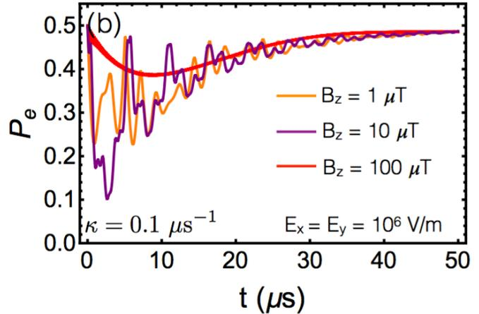
Figure 2: Error probability,  $P_e$ , as a function of time for three different applied magnetic fields. Measurements of the POVM should take place at times and magnetic fields where  $P_e$  is minimum (around 3 microseconds and 10 microtesla).  $\kappa$  is the decoherence rate.
