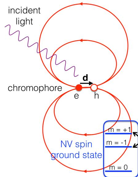
Figure 1: Model of photon detection. Dynamic charge polarization is detected by the NV center through spin transitions (black double arrow).
