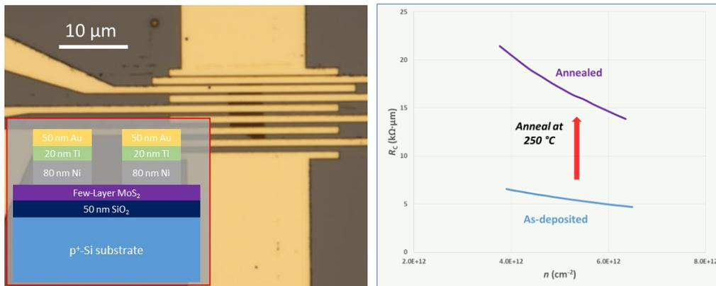
Figure 1. (a) Optical image of a TLM test structure; (inset) schematic of a back-gated MOSFET with Ni contacts. (b) Contact resistance for as-deposited and annealed Ni contacts versus sheet carrier density ( $n$ ).
