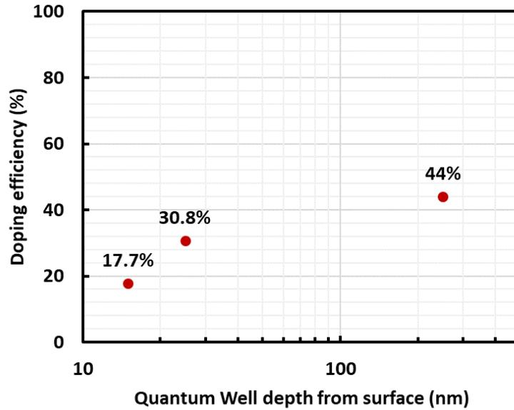
Fig. 2. Plot of doping efficiency of n-type Silicon dopants vs. depth of a 25nm wide InAsSb QW on GaSb substrate. As the QW is brought closer to the surface, the doping efficiency reduces, indicating the presence of a surface depletion layer (negative charges). This would indicate the fermi-level at the surface is pinned within the gap of the semiconductor.
