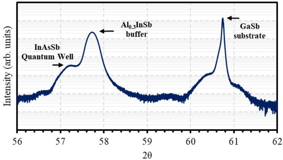
Fig. 3. X-Ray diffractogram of an InAsSb QW grown on an  $Al_{0.3}InSb$  barrier layer on a GaSb substrate. The diffraction peak for the QW corresponds to a composition of  $InAs_{0.2}Sb_{0.8}$ . This diffractogram in conjunction with *in-situ* Reflection High Energy Electron Diffraction (RHEED) indicates that the quantum well is strained compressively on the  $Al_{0.3}InSb$  buffer/barrier layer.
