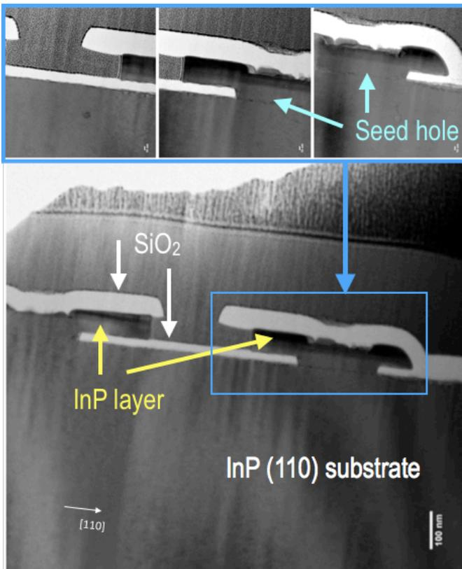
Figure S2 Cross-sectional TEM images of epitaxial InP layers grown inside the confined structure. Growth fronts toward the feed hole show the desired vertical facet. The depth of seed hole (i.e. thickness of bottom SiO<sub>2</sub> layer) is 20 nm and the height of tunnel is 50 nm.
