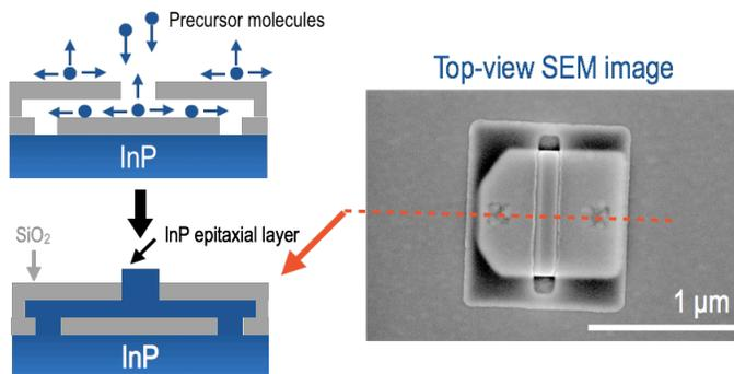
Figure 1 The confined structure is defined by SiO<sub>2</sub> horizontal and vertical layers. Precursor molecules, trimethyl-indium and thermally cracked phosphine enter into the structure through the feed hole in the center and arrive onto the two seed holes where the growth initiates. Top-view SEM image confirms the epitaxial growth inside the confined structure.
