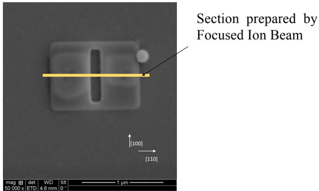
Figure S1 Top-view SEM image showing the section used for cross-sectional TEM analysis.
