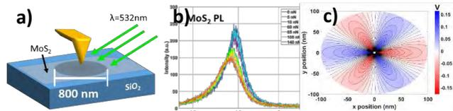
Figure 1: (a) Schematic depicting indentation and PL characterization. (b) PL measurement of MoS<sub>2</sub> during indentation. (c) Calculated electrostatic potential from piezoelectricity in indented MoS<sub>2</sub>
