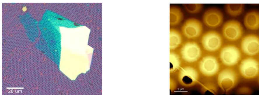
**Figure S1.** a) Optical image and b) AFM image of exfoliated MoS2 transferred onto SiO2 substrate with nanopatterned holes.
