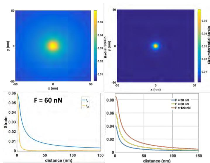
**Figure S2.** Calculation of the strain distribution of a circular membrane of 500nm diameter MoS2 indented by a spherical indenter of radius 7nm. The top panels are contour plots of the distribution of a) radial and b) circumferential strain for 60 nN of indentation force. The majority of strain is confined to a very small area near the point of indentation. Profiles of the contour plots along the x-axis are shown in c), while d) shows the dependence of the strain on indentation force.
