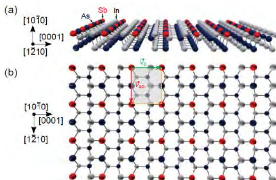
Figure 1 Perspective view of a ball model of the two-dimensional idealized (long range) chemical ordering of the monolayer shell on the InAs sidewall facet, based on the ordering and antiordering vectors extracted from pair correlation function. (a) Side and (b) top view with surface unit cell.
