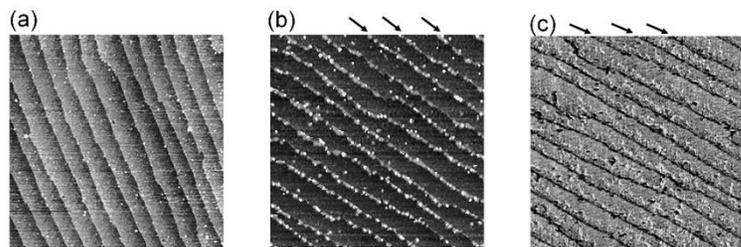
Figure 1. AFM images ( $1 \times 1 \mu m^2$ ). After (a) first, and (b) second LOW treatment, respectively. (c) After subsequent etching of a sample in (b) in HF and  $H_2O_2$ .
