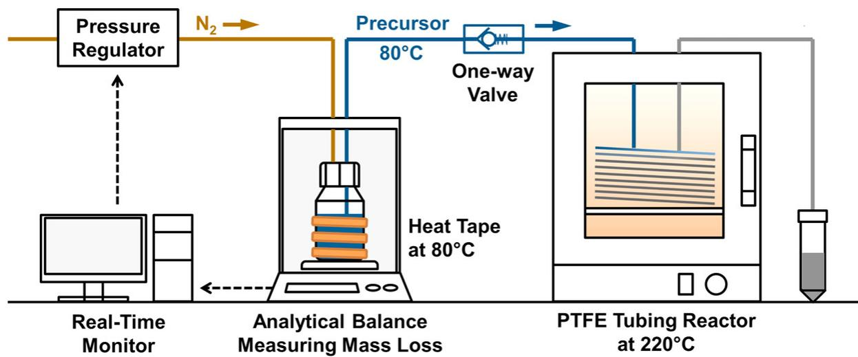
**Figure 1.** Representative continuous flow nanofabrication device
