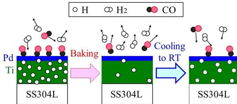
Fig 1. Schematic of the activation and pumping mechanisms of oxygen-free Pd/Ti thin film [2].
