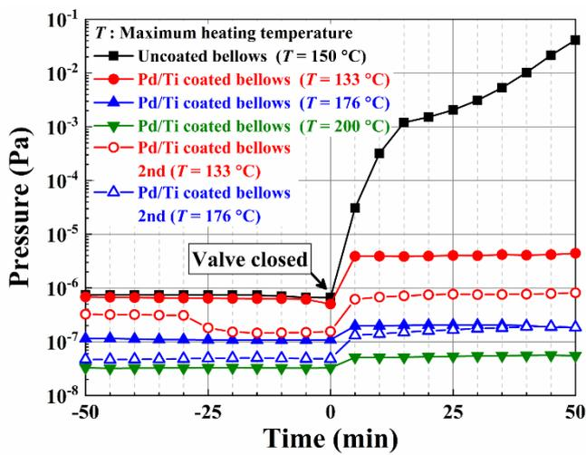
Fig. 2 Summarized pressure curves of uncoated bellows and oxygen-free-Pd/Ti-coated bellows [1].
