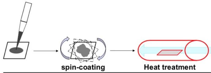
Fig. 1. Molecular precursor method (MPM).
