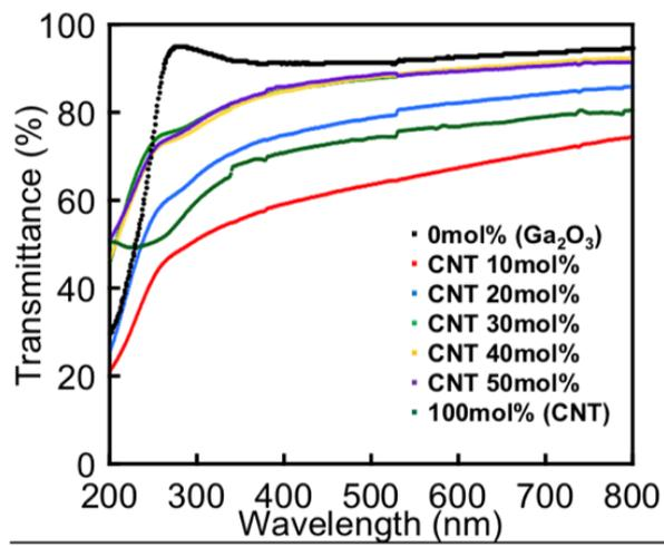
Fig. 3. Transmittance spectra of CNT doped Ga<sub>2</sub>O<sub>3</sub> thin films at RT.
