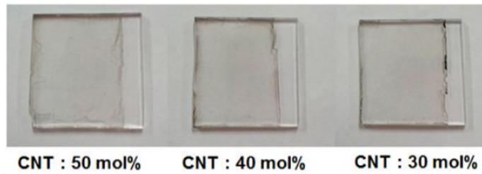
Fig. 2. CNT doped Ga<sub>2</sub>O<sub>3</sub> thin films
